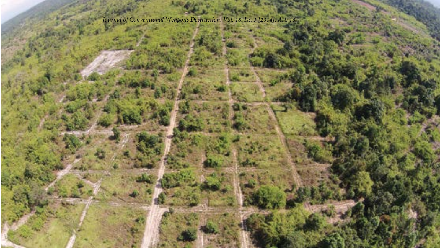
In Phase 2, lanes are cut every 25 meters, perpendicular to each other to form a grid. Photo courtesy of HD R&D.
