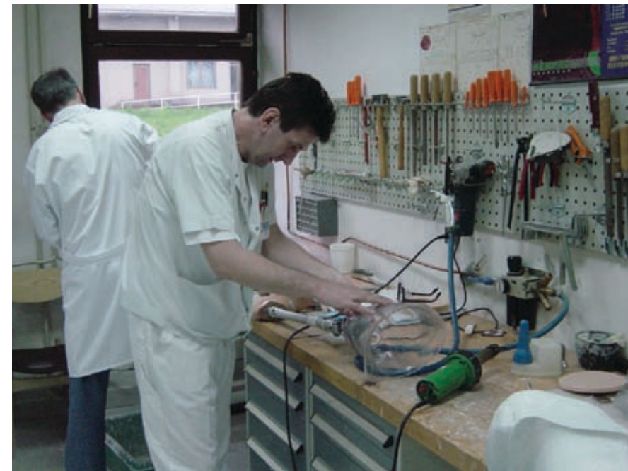
Student in the CIR's distance learning program working on a transtibial socket during the ISPO practical exam.
