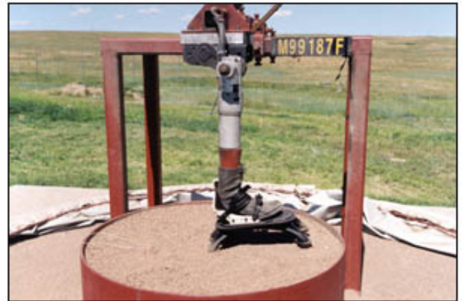
Instrumented mechanical surrogate leg used in DRES tests.
