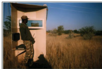
Protective Blast Shield.
