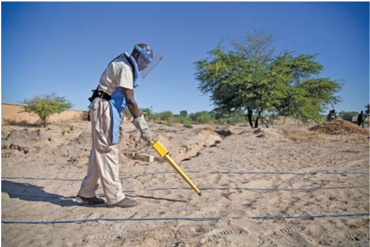
An operator with The Development Initiative uses a magnetic locator to conduct battle area clearance activity at the Malian army camp in Timbuktu, December 2013. Photo courtesy of UNMAS.
