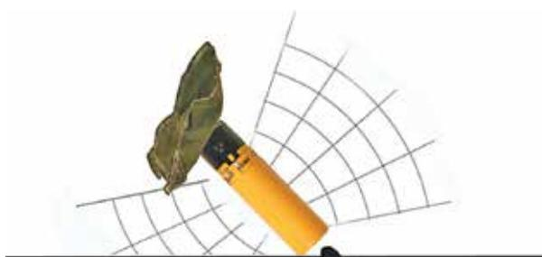
Figure 4. Probable fragmentation dispersion for a BLU-97 submunition on a flat hard surface. Note the fragmentation pattern is broadly similar to a fin-stabilized submunition, but the shaped charge will likely produce a larger hole or scabbing at the base of the pattern.
