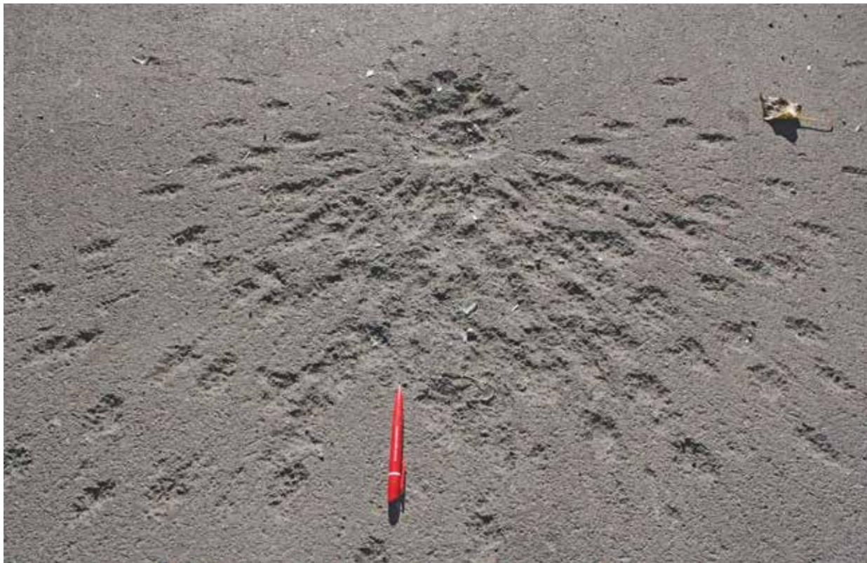
Image 4. Fragmentation pattern on a hard surface caused by a 9N210 submunition impact outside ICRC office on Universitetskaya Street, Donetsk, October 2014.
