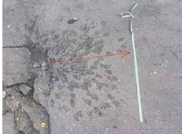
Image 11. 9N210 fragmentation pattern, Donetsk, Ukraine, October 2014. The superimposed line indicates the direction from which the submunition impacted. Photo courtesy of Harriet Salem.
