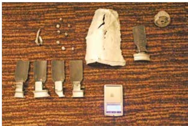
Image 6. Fragmentation from a 9N210 submunition collected at the scene of a cluster munition strike in Donetsk, October 2014. It is important to try to corroborate submunition impact patterns with associated fragmentation when possible.
