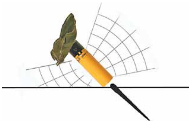
Figure 4. Probable fragmentation dispersion for a BLU-77 submunition on a flat hard surface. Note the fragmentation pattern is broadly similar to a fin-stabilized submunition, but the shaped charge will likely produce a larger hole or scarring at the base of the pattern.
