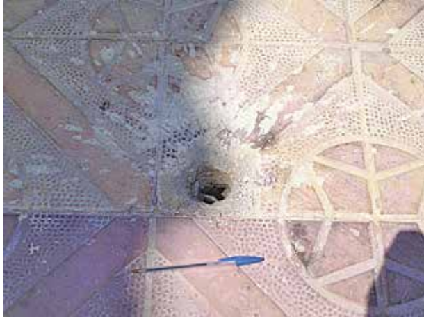
Image 8. M Series DPICM impact pattern on a tiled hard surface, showing the central hole made by the shaped charge, southern Lebanon, August 2006. Note that the fragmentation pattern is broadly similar to a fin-stabilized submunition, but the shaped charge will likely produce a larger hole at the base of the pattern. Photo courtesy of Steve Priestley.
