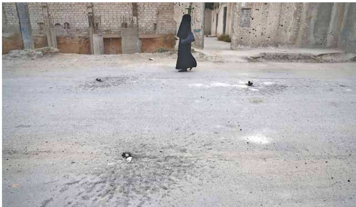
Image 7. Mortar impact patterns, Douma, Syria. Note how the scarring is similar to cylindrical submunition fragmentation patterns. The two are easy to mistake for one another. Also note the same orientation of the three patterns indicating they all came from the same direction and probably from the same mortar barrel. The mortar round tail units are embedded at the base of each pattern. Photo courtesy of KiloBuzz.
