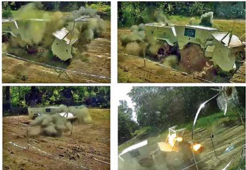
Stills from a video of the testing using real mines.<sup>14</sup>
