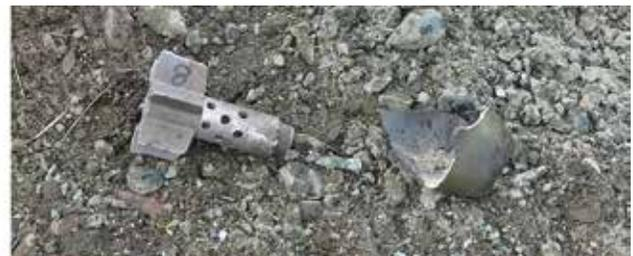
New liner three: in both mortars, the HE burned to deflagration.
