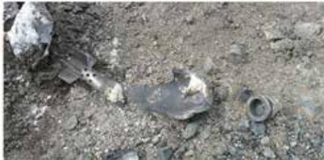
Burned out mortar shell (left) and deflagrated munition (right).
