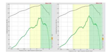
**Figure 3:** Starkey programming software: Predicted real ear measures (dB SPL) represented by the solid green line as a function of frequency (Hz). Right panel: Spectral iQ on, Left panel: Spectral iQ off.
