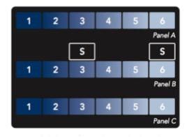
**Figure 1:** Spectral iQ. Panel A depicts traditional amplification from a hearing aid utilizing 6 channels. Panel B: shows Spectral iQ activated and transposing the /s/ phoneme. Panel C represents the hearing aid reverting back to traditional amplification when no high frequency stimulus is detected (Galster et al., 2011)
