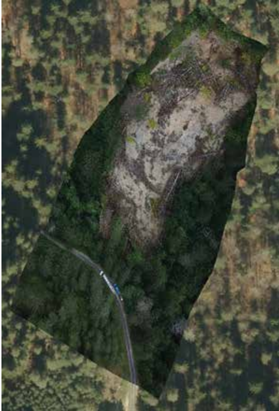
Image 5. The landslide Olovskie luke, a digital orthomosaic derived from the aerial images collected 27 August 2014 by RPAS after floods, overlaid on digital orthophoto map produced in 2013, before floods.
