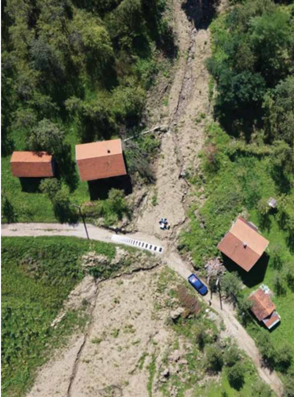
Image 4. Example of the landslide, which crosses the minefield in the upper part. A digital orthomosaic derived from aerial image collected by RPAS.
