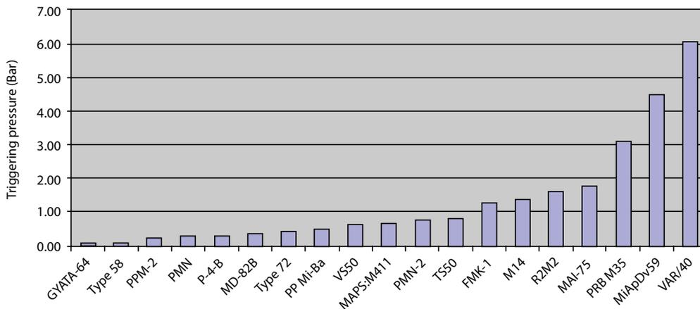
Figure 1: Triggering pressure for various AP landmines.
