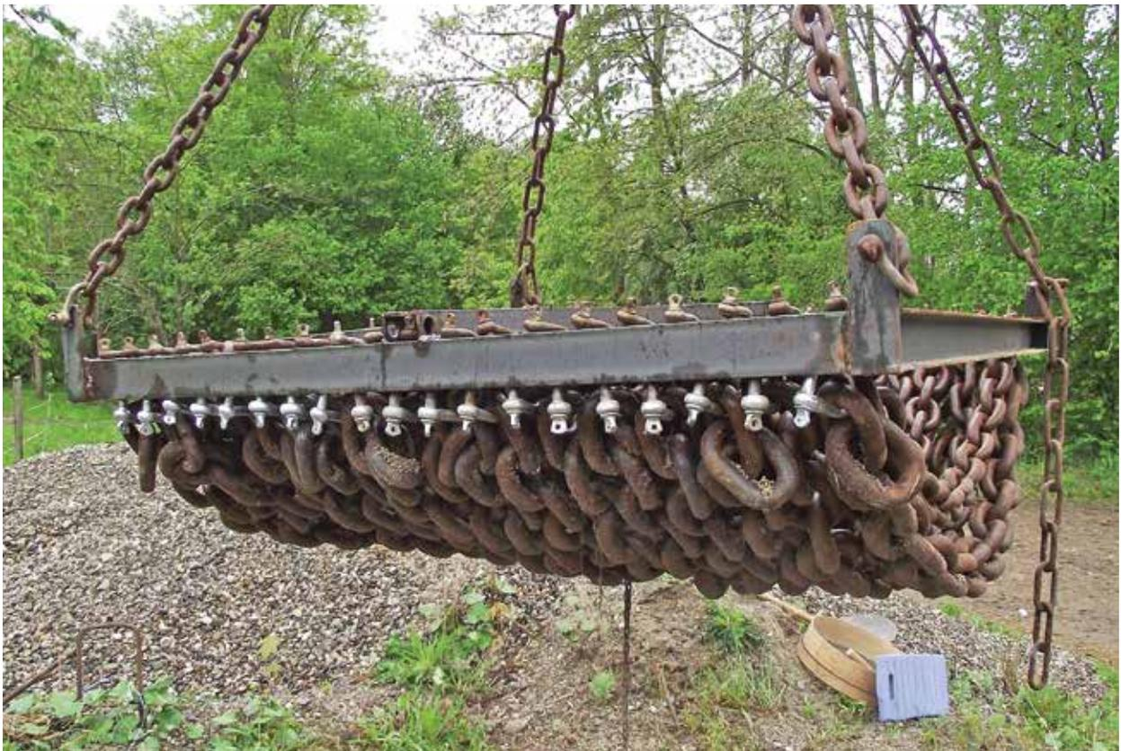
High mass density chain arrays used during testing.
