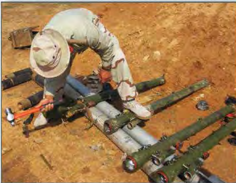
A member of the Quick Reaction Force disables loose and at-risk MANPADS before the missiles' eventual destruction. Photo courtesy of the Quick Reaction Force.
