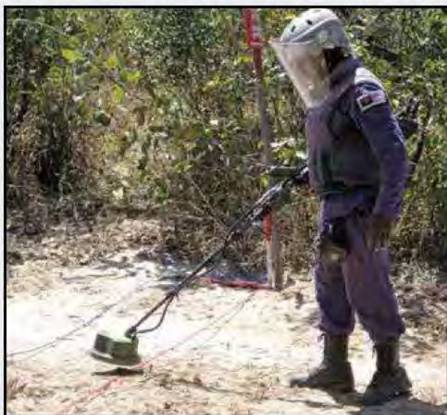
A U.S.-funded MAG deminer uses a U.S. DOD Research and Development Night Vision and Electronic Sensor Directorate, or NVESD, dual-purpose mine detector in Luena, Moxico, Angola. Photo courtesy of Darren Manning, PM/WRA, U.S. Dept. of State.
