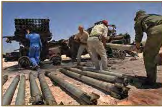
MAG Technical Field Manager and Team Leader Fred Gras unloads a BM-21 Grad rocket launcher in Adjadabya, Libya. The launcher had been hit in a NATO airstrike and still contained 15 fuzed 122 mm rockets.
