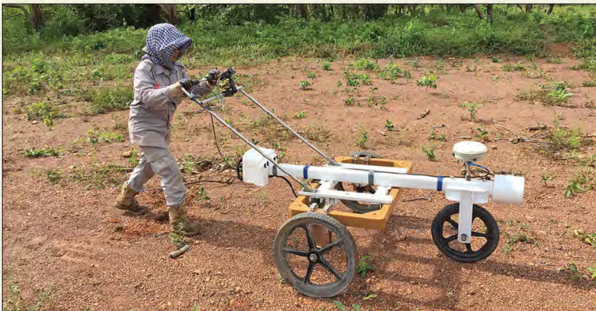
MAG deminer uses the HD R&D Program's Scorpion system to detect UXO in eastern Cambodia. Photo courtesy of HD R&D.
