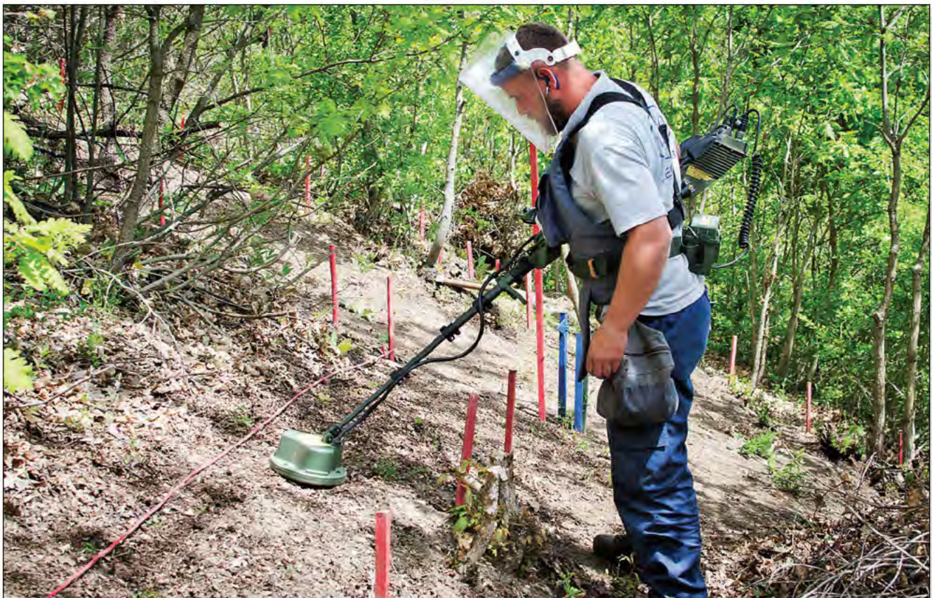
A HALO deminer operate the HD R&D Program's HSTAMIDS in Kosovo. Photo courtesy of HD R&D.
