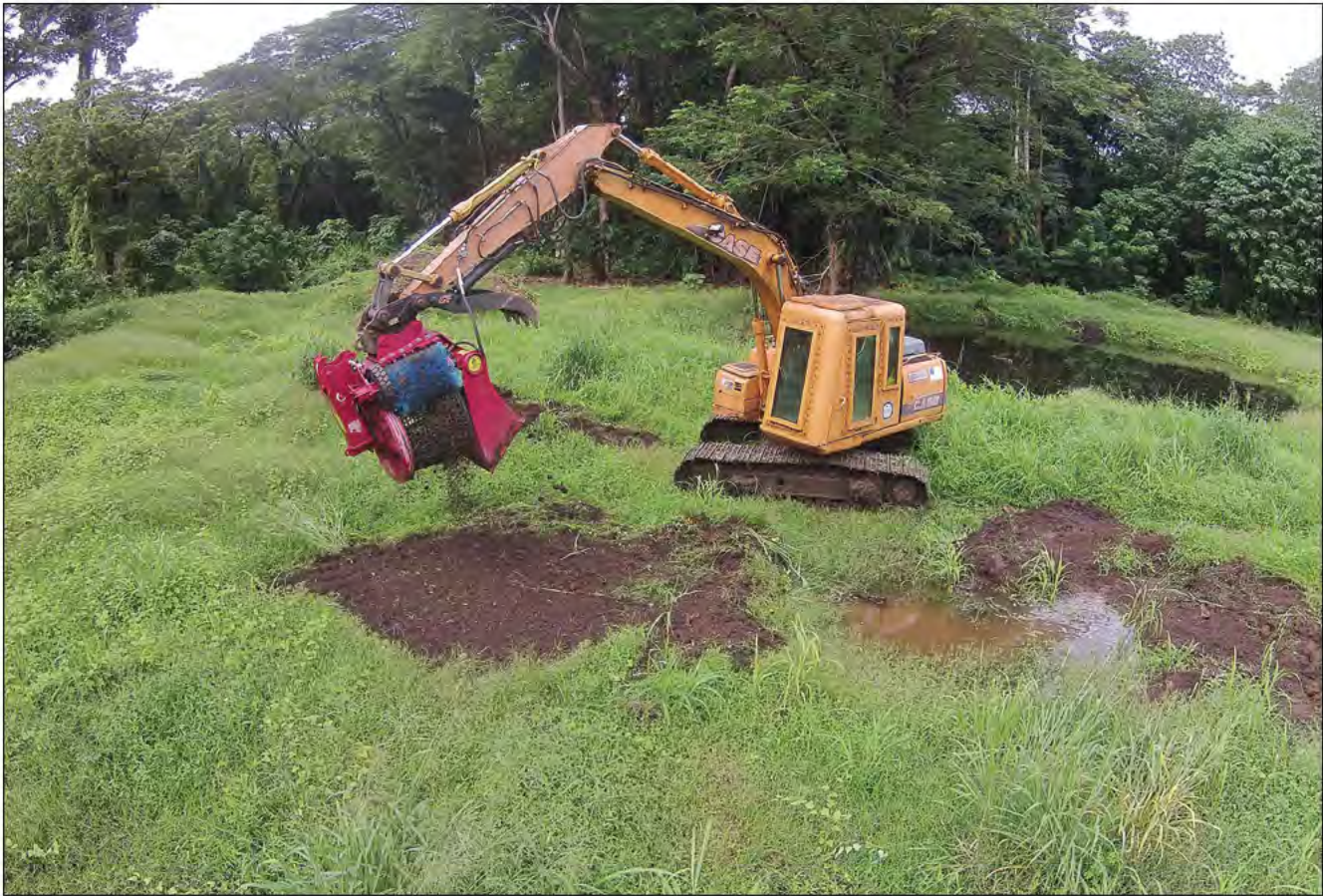
The Royal Solomon Islands Police Force operates a tool provided by the HD R&D Program to find UXO in water-laden soil. Photo courtesy of HD R&D.
