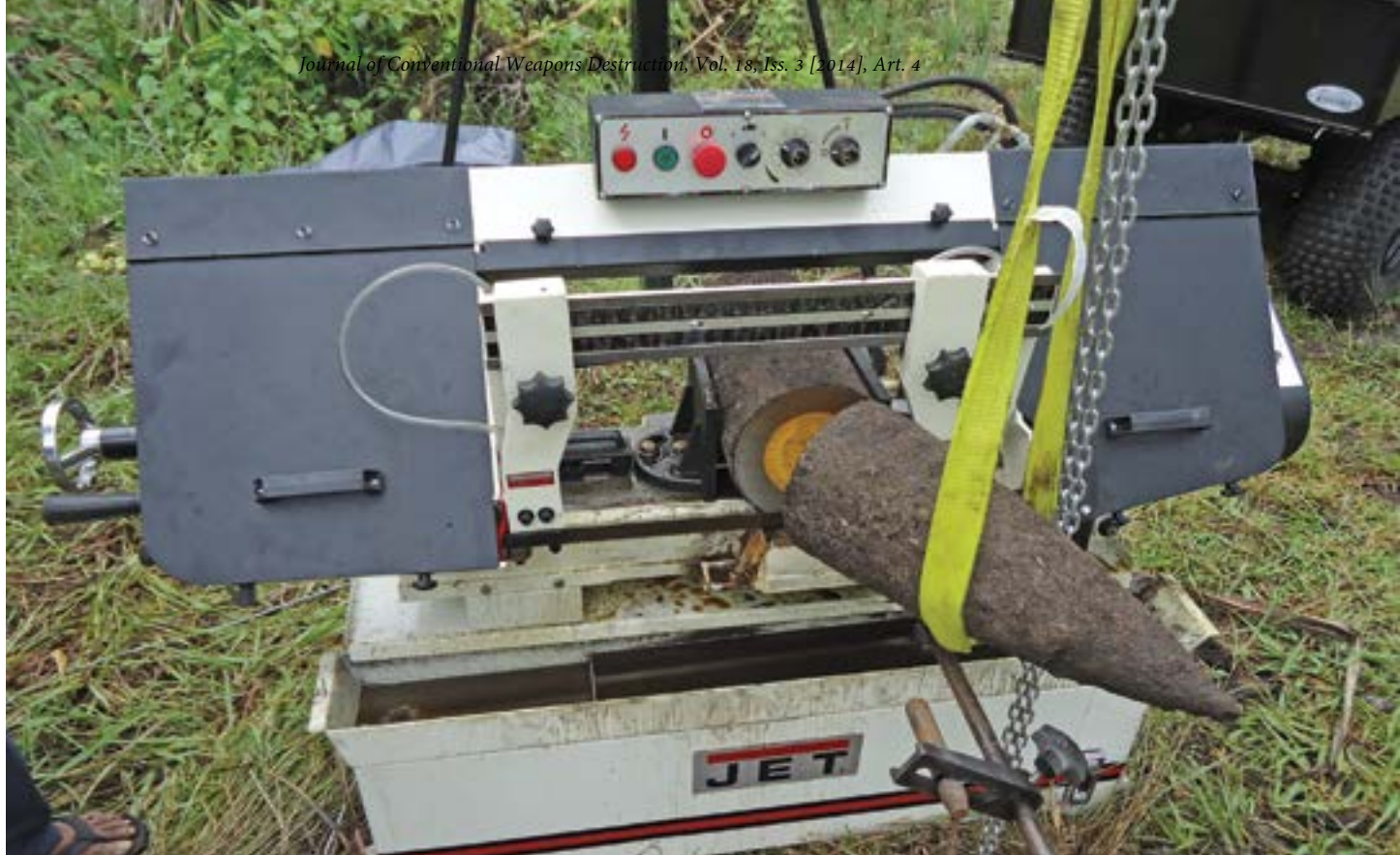
Golden West's Mobile Bomb Cutting System.
