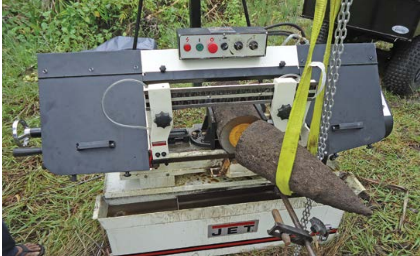
Golden West's Mobile Bomb Cutting System.
