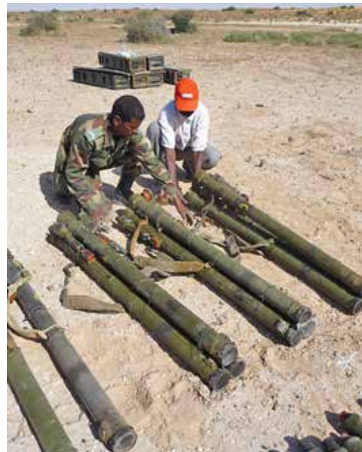
Preparation of and grouping of MANPADS for destruction.
