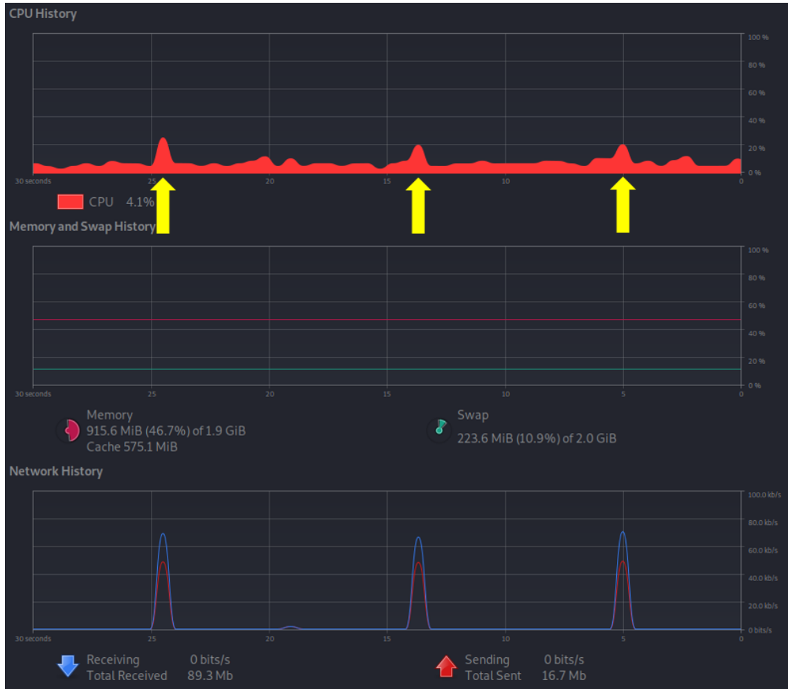
Figure 5.11: CPU usage for submission using multithreading.
