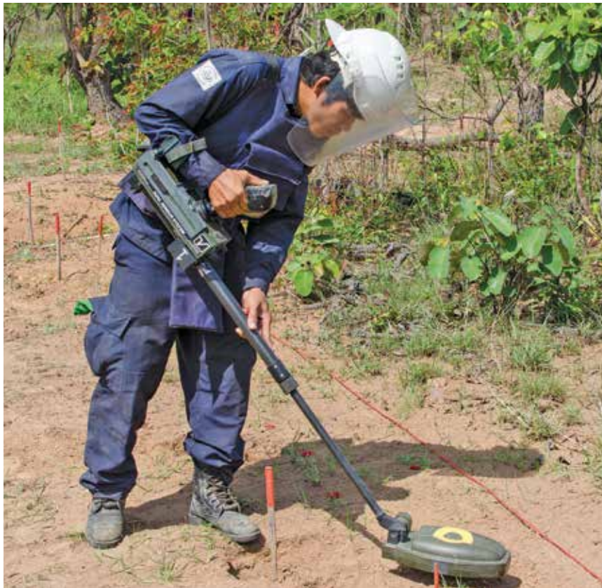
A MINEHOUND VMR2 is used to find AP mines in Cambodia. The use of this system allows 92% of signals from metallic rubbish to be rapidly excavated.
