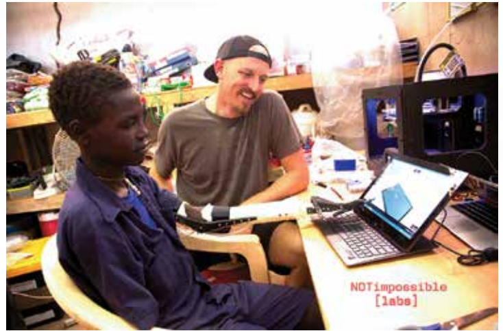
Mick Ebeling (right), CEO and Founder of Not Impossible Labs, with Daniel Omar (left) wearing a prosthetic arm created with Not Impossible Labs 3-D printing technology. Photo courtesy of Not Impossible Labs.
