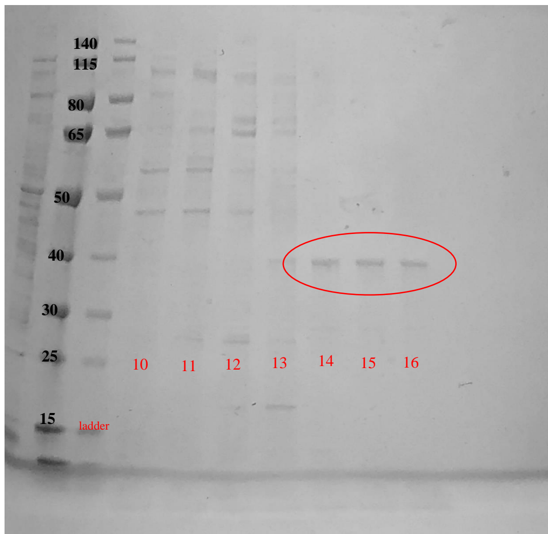
Figure 7. SDS PAGE gel from FPLC purification of wild type Uba5 using 1 mL HisTrap TM HP nickel column. Shown on the left is PageRuler Prestained Protein Ladder with markers for each molecular weight in units of kD. Marked in red are fractions from the purification described in Figure 6. Bands corresponding to Uba5 are circled in fractions 14, 15, and 16.
