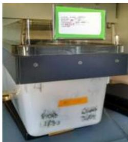
**Figure 1. Cage Top Warmer.** The gray piece on top of the cage is the warm air circulator, which lies below the HEPA filter. It maintains  $T_{amb}$  within strict limits for the duration of the recovery period.
