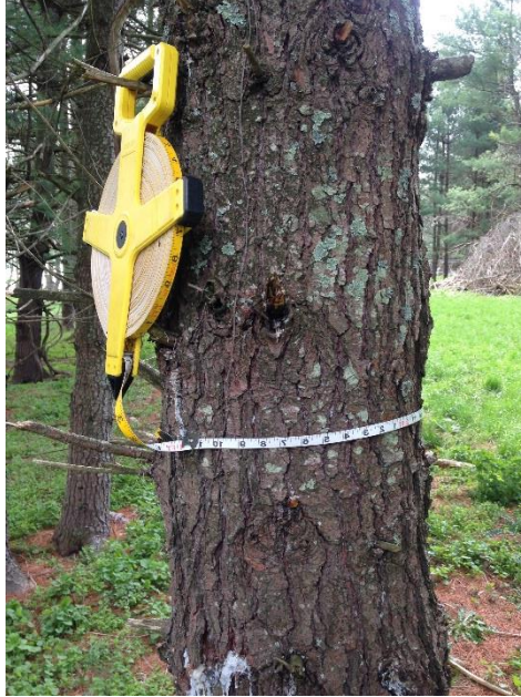
Image 4. Measurement Method for Tree Circumferences.
