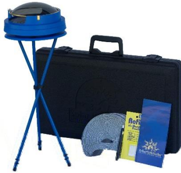
Figure 10. Solar Pathfinder Kit (Solar Pathfinder, 2015)
