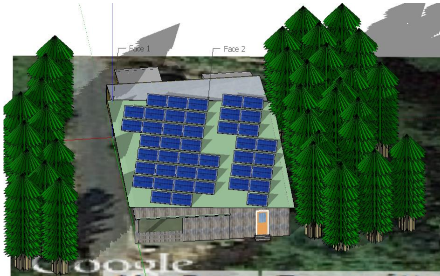
Figure 12. Roof Mount Solar PV System Rendering.
