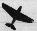
A PURSUIT PLANE, at a cruising speed of 200 m.p.h. requires one gallon of gasoline for every four miles of flight.
