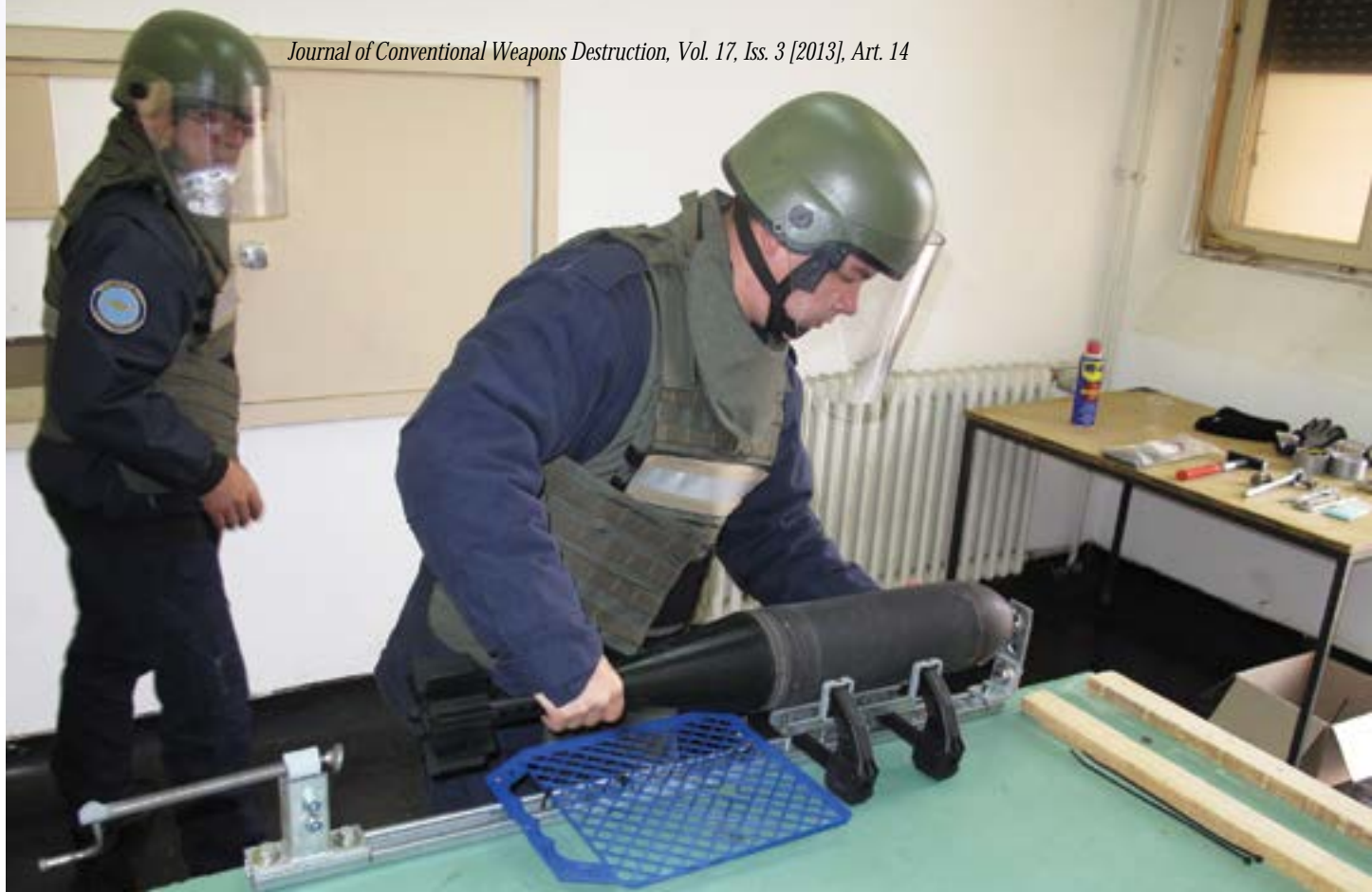
Example of in-country solutions: A Macedonia M93 mortar disassembly using locally procured tools with low-tech specialty equipment.
