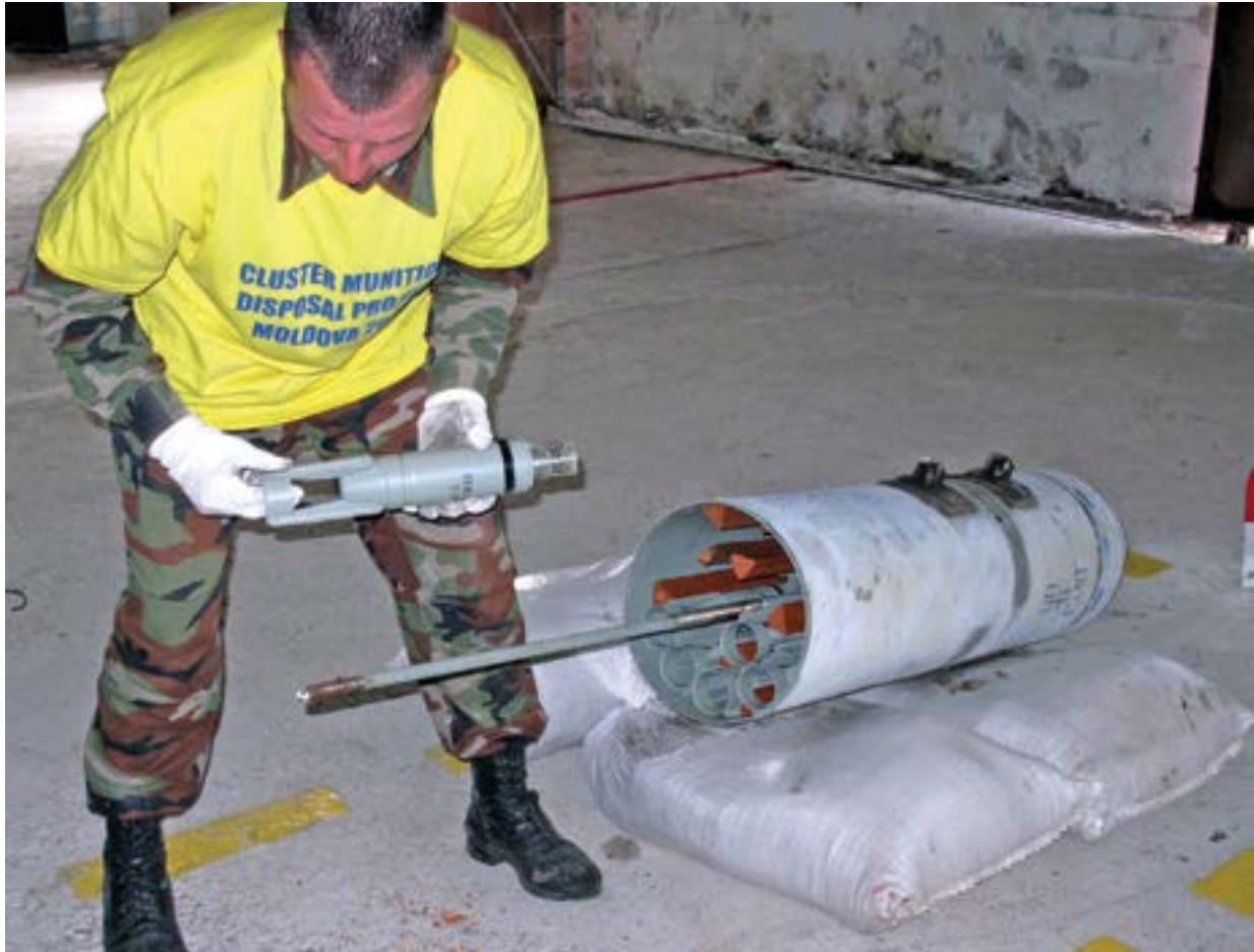
Norwegian People's Aid trained Moldovan civilians in the Moldova project. In this photo, PTAB 2.5M submunitions are extracted from an RBK dispenser. Photo courtesy of Werner Anderson.
