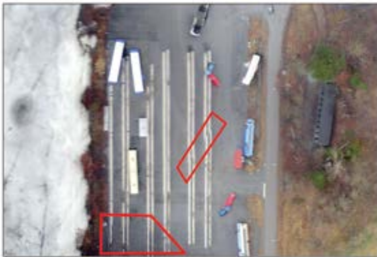
Figure 8. Line and object deformations in orthoimages. Figure courtesy of GICHD.
