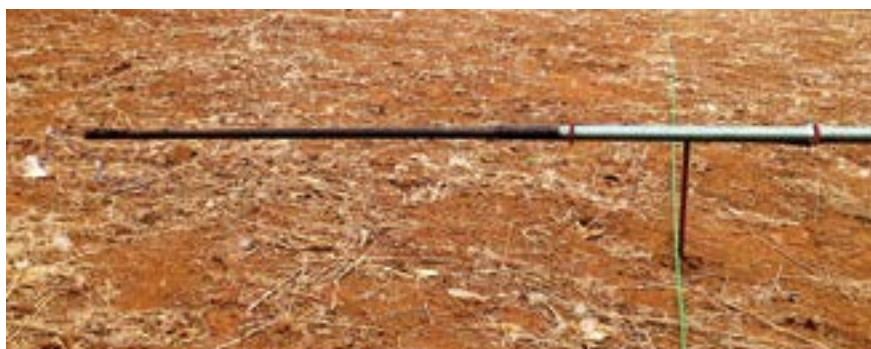
The fishing rod apparatus used to place a TNT-filled bag inside the search area.
