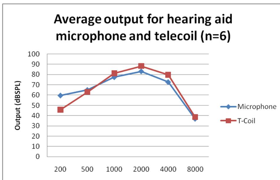
**Figure 4.** Shows the average output (dB SPL) for the subjects' hearing aid microphone (60 dB SPL input) and t-coil (31.6 mA/m input) using ANSI S3.22.
