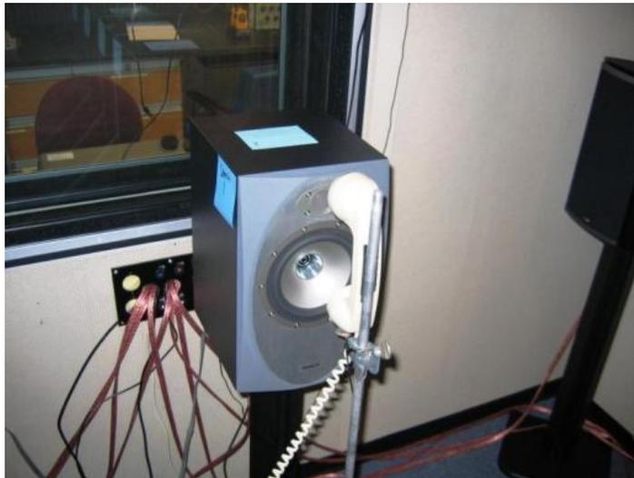
**Figure 2. Standard landline telephone handset placed 6 inches from main driver of Tannoy 600 speaker.**
