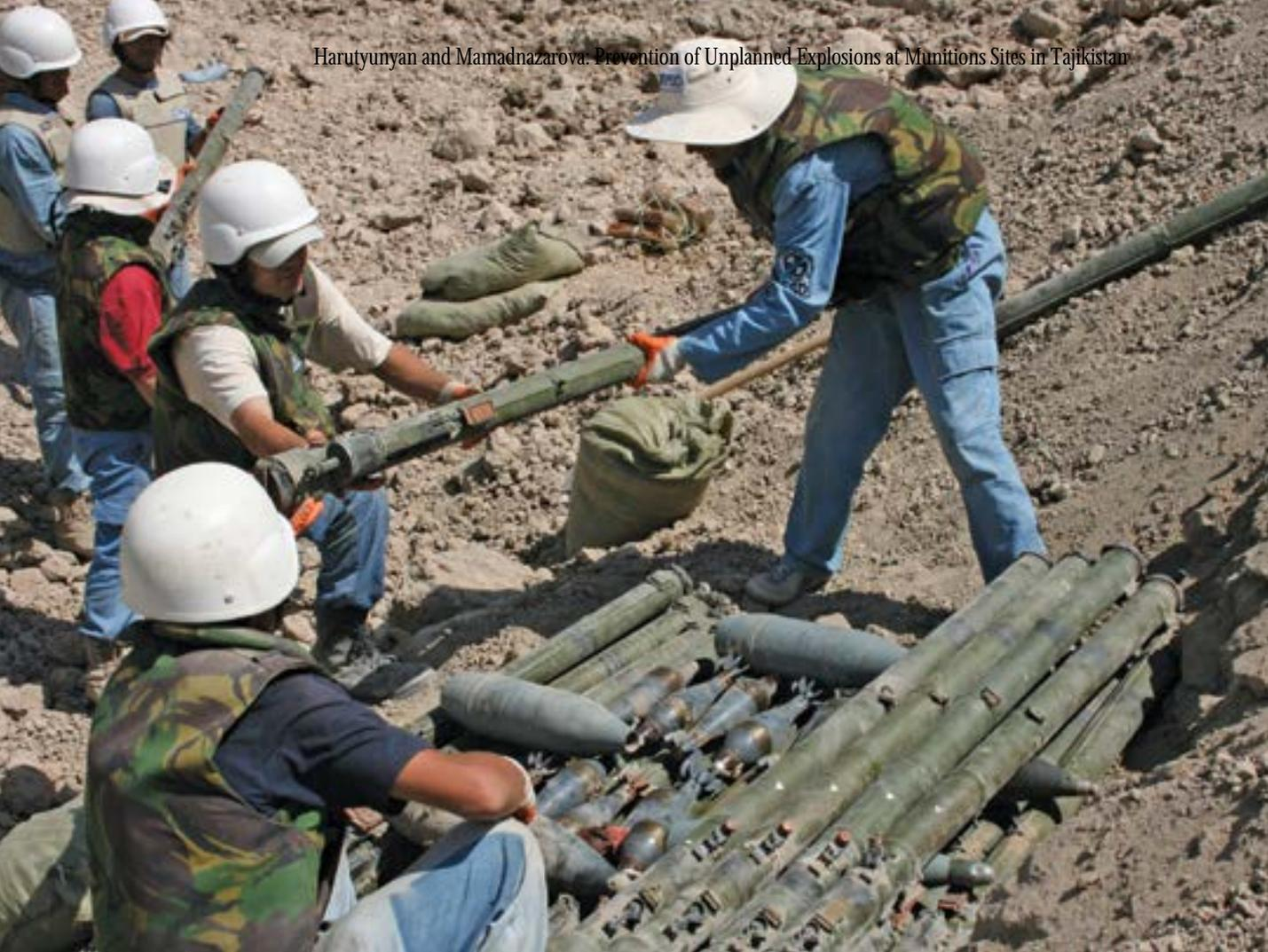
Demolition pit with MANPADS, mortar shells and artillery shells.
