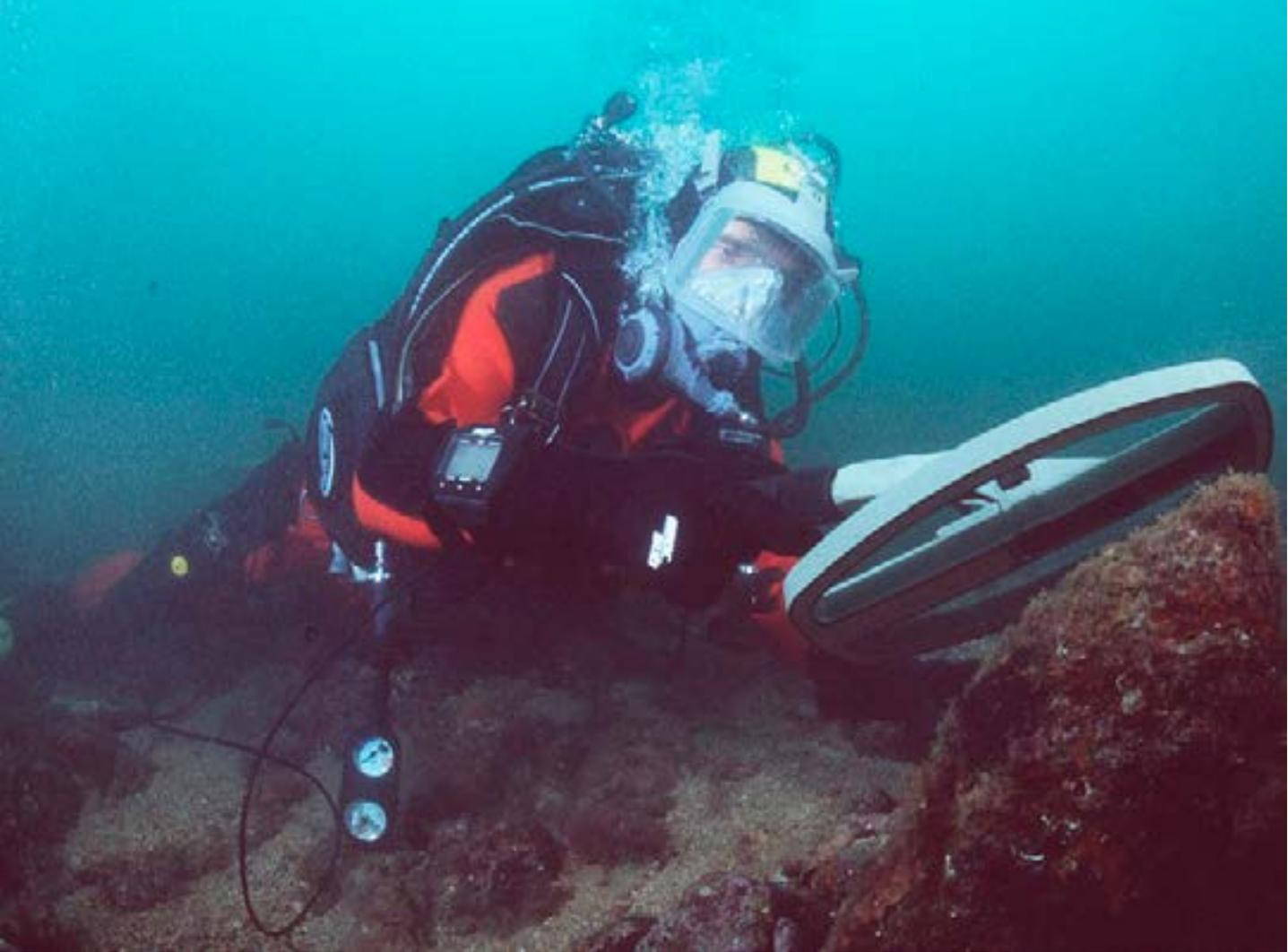
A diver uses an underwater metal detector produced by Vallon to perform underwater mine reconnaissance of the seabed in the Bay of Kotor, Montenegro.
