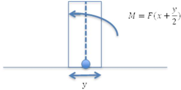
Figure 20: re-simplified model of clip attachments
