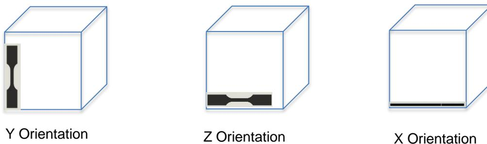
Figure 32: Orientation of Specimens
