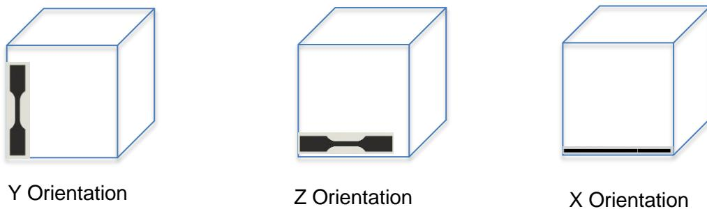
Figure 32: Orientation of Specimens
