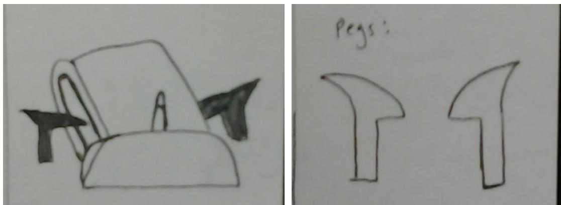
Figure 8: Clip attachments conceptual design
