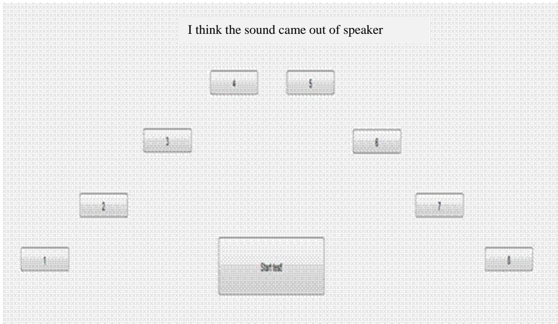
Figure 2: Screenshot of the sound localization testing screen used by the subject to indicate the perceived speaker location of the broadband noise stimulus on an azimuth plot on the computer screen.
