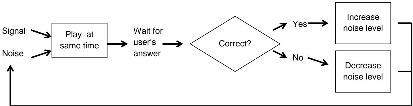
Figure 9: Design of Speech in Noise Hearing Test (excludes Training Loop)
