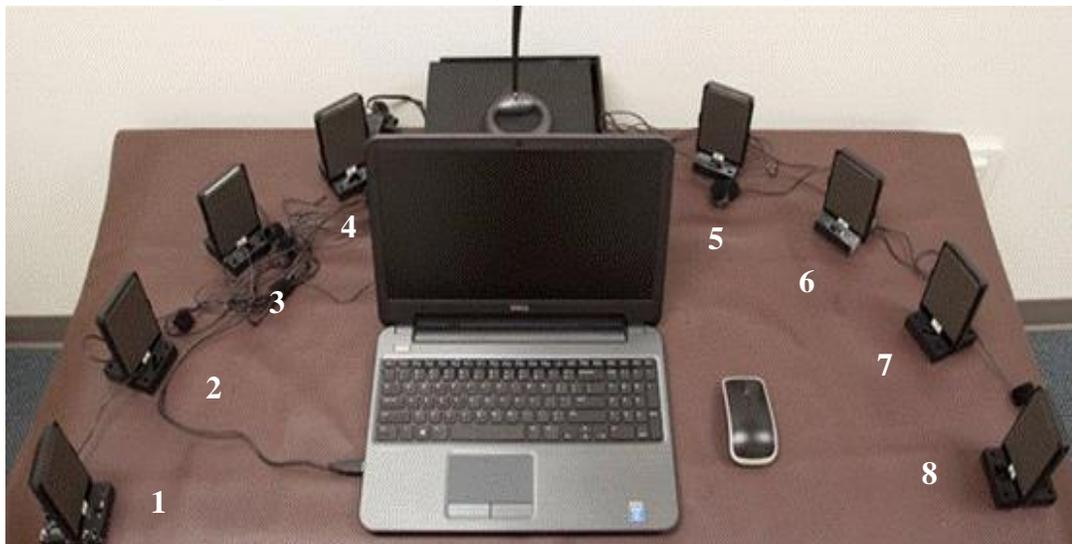
Figure 1: The laboratory-made stereo-hearing device used to test all subjects in the binaural processing tasks of sound localization and understanding speech in noise. The device set-up contains a laptop, custom table-mat with 3-D printed speaker stands, and 8 speakers (labeled 1 to 8 from left to right) precisely placed in a 180-degree azimuth.
