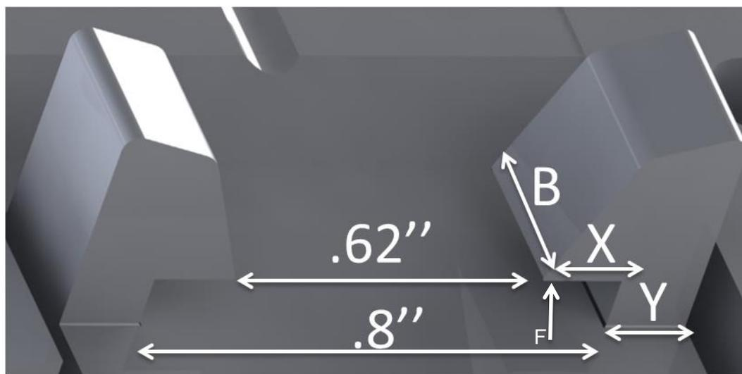
Figure 37: Dimensions of Speaker Hooks
