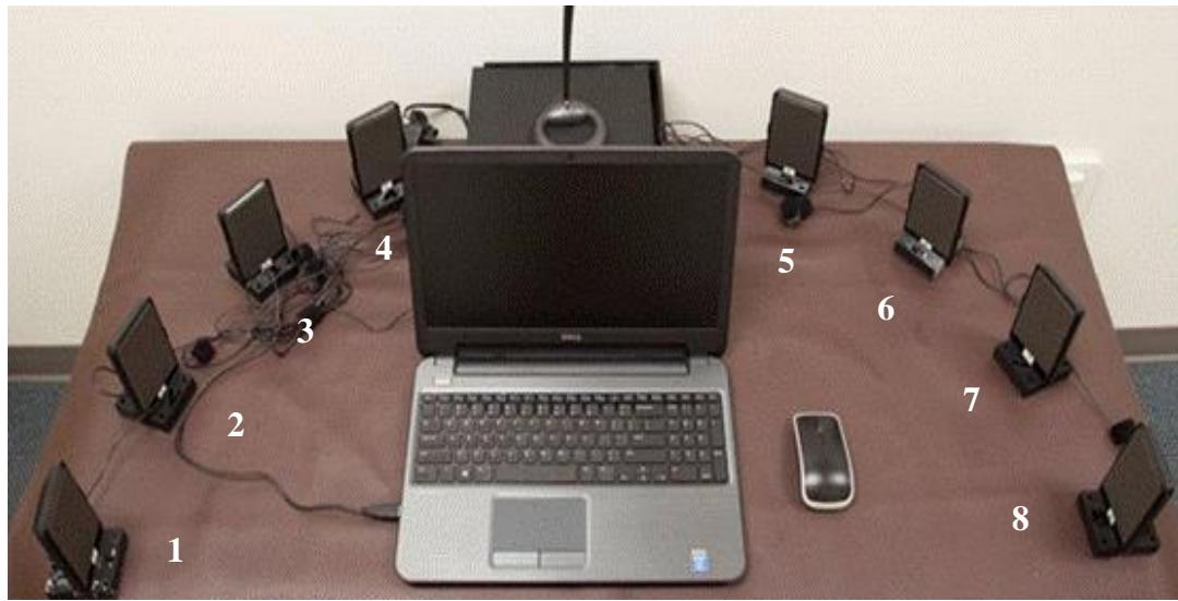
Figure 1: The laboratory-made stereo-hearing device used to test all subjects in the binaural processing tasks of sound localization and understanding speech in noise. The device set-up contains a laptop, custom table-mat with 3-D printed speaker stands, and 8 speakers (labeled 1 to 8 from left to right) precisely placed in a 180-degree azimuth.
