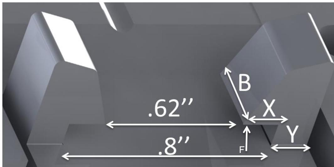
Figure 37: Dimensions of Speaker Hooks
