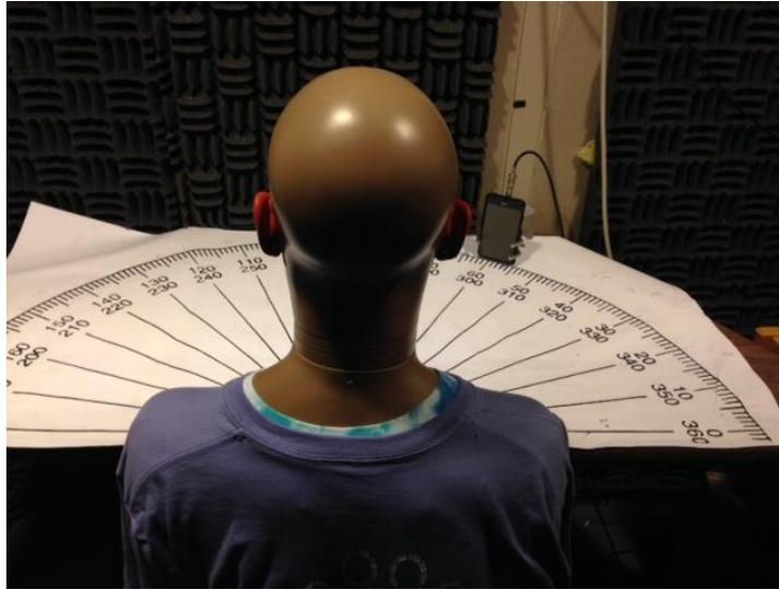
Figure 35: KEMAR Experimental Set Up
