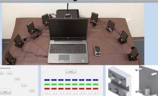
Figures above show the assembled system (top), screen shots from the sound localization and speech-in-noise tests (bottom left and center), and the 3D printed pieces to hold the speakers (the 'male' part is glued to the mat), and the fitting piece is clipped to the appropriate speaker for easy, fool-proof setup.
