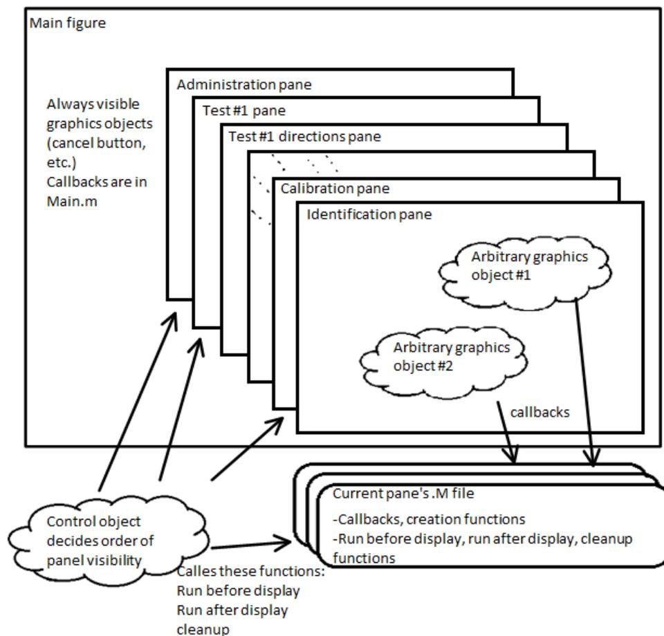
Figure 7. Framework used in the GUI. Any number of uipanelns can be added to allow addition of another audio test, more instructions, etc.
