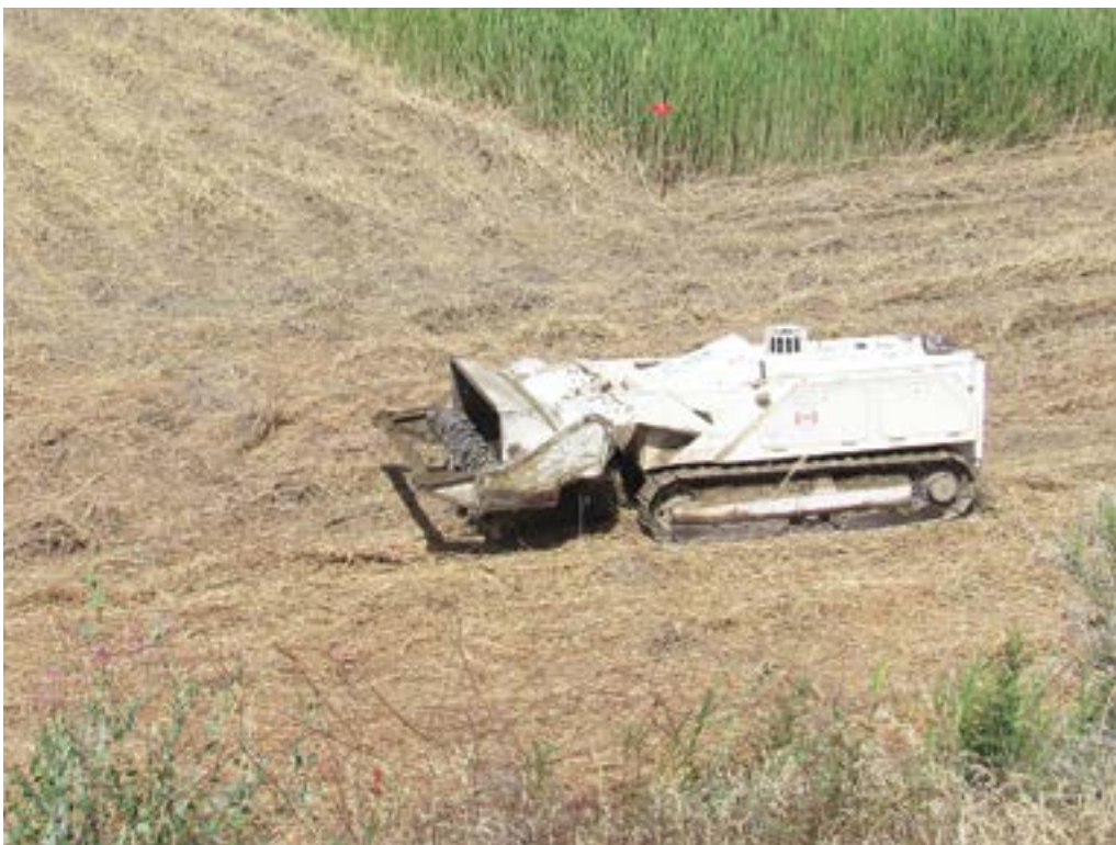
Medium flail used for vegetation cutting, ground preparation and possibly mine detonation.
