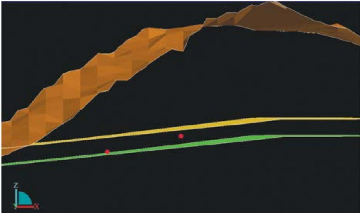
Figure 3. A 3-D model of the brown present surface seen together with the position of the hazard layer outlined by the yellow and green surface inside a dune. The hazard layer is 1.9 m wide and the position of the two mines is seen inside the defined hazard layer. The sand above the yellow top of the hazard layer could be excavated without prior mine clearance.
