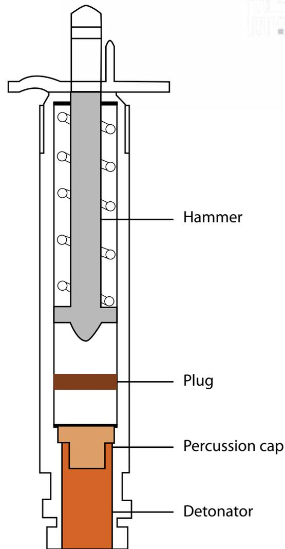
Figure 5. Schematic illustration of the Z.Z.42 fuze. The dimension is approximately 1.2 x 8.5 cm. Notice the position of the plug, which is composed of a mixture of sand grains, oil and rust.
