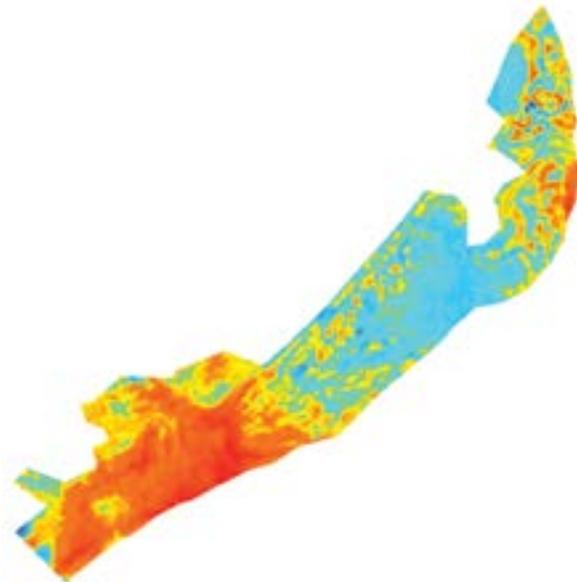
Figure 2. Digital differential model of the marsh covered with dune. Size of the area is 57,740 sq m. Red indicates areas where the hazard layer is situated inside the dune. Blue areas indicate where the hazard layer is part of the present surface. Approximately 30,000 cubic meters could be excavated without clearance.
