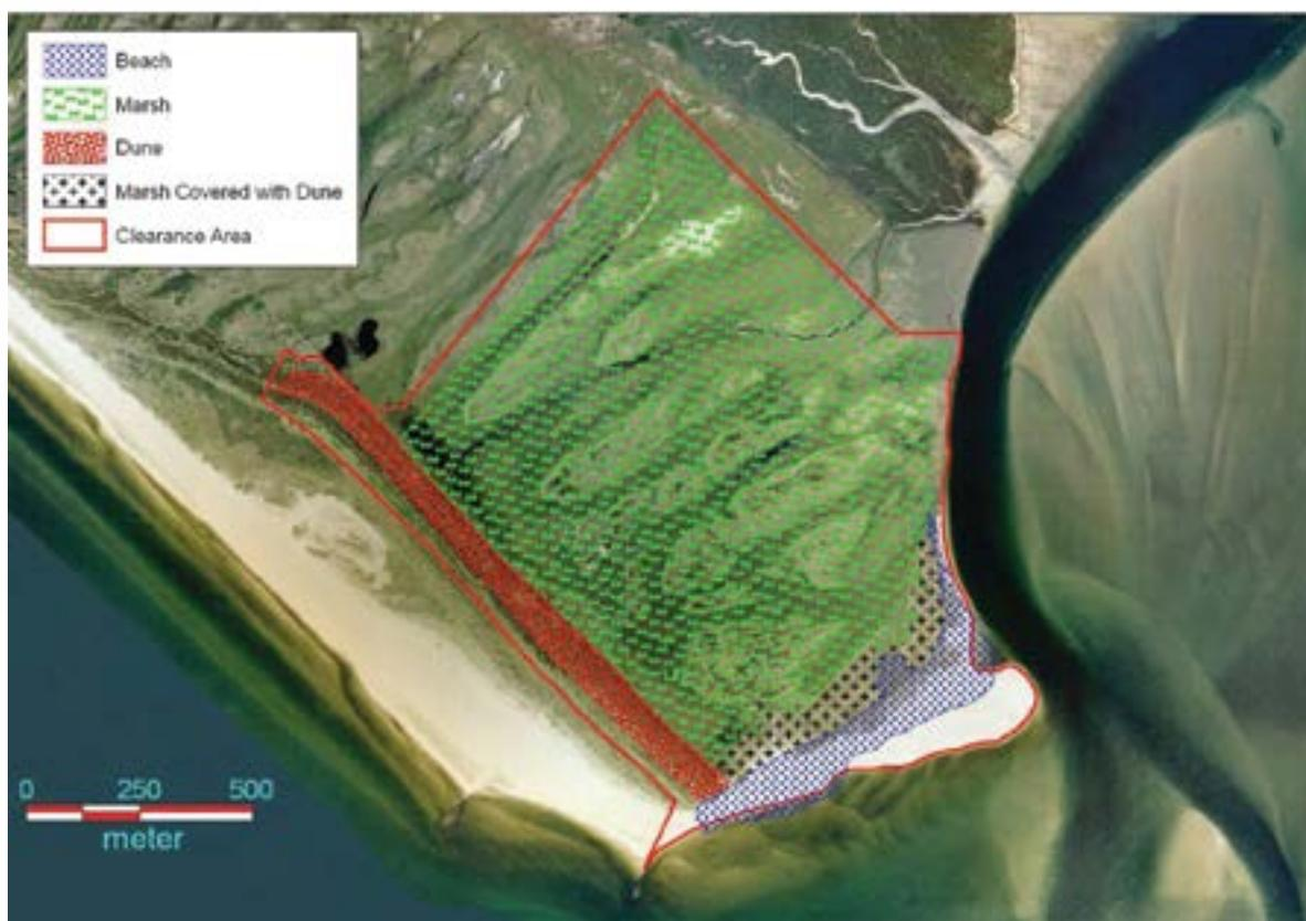
Figure 4. Figure 4 shows the new division of the area after evaluating terrain and digital-terrain model. The dune area was divided into two areas by reducing the mined volume to be cleared. See Figure 1 for comparison.
