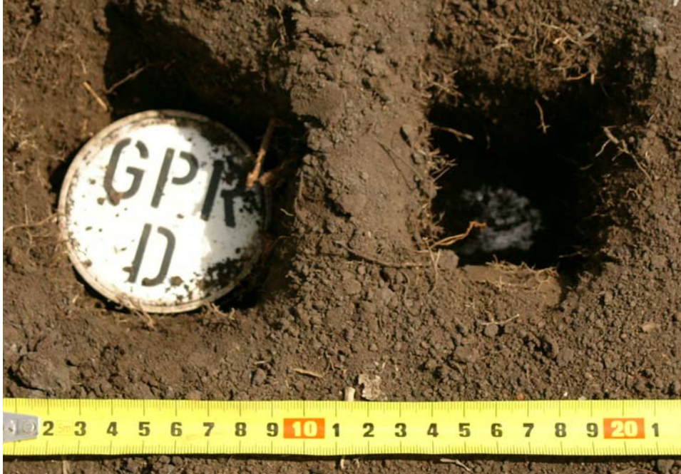
Figure 5 Buried metal disc and ERA test piece for the resolution of adjacent targets test
