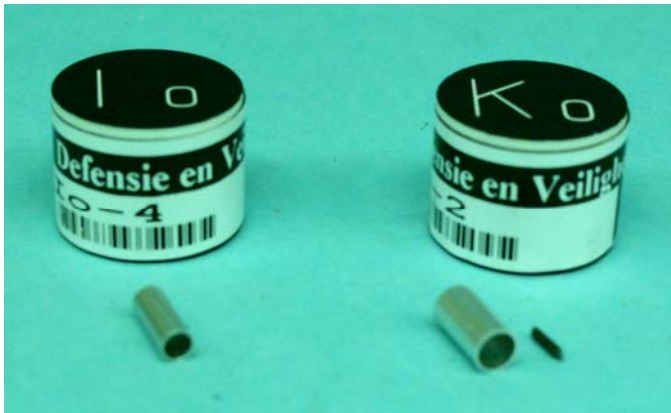
Figure 2b ITOP inserts Io and Ko with their metal parts in front.
