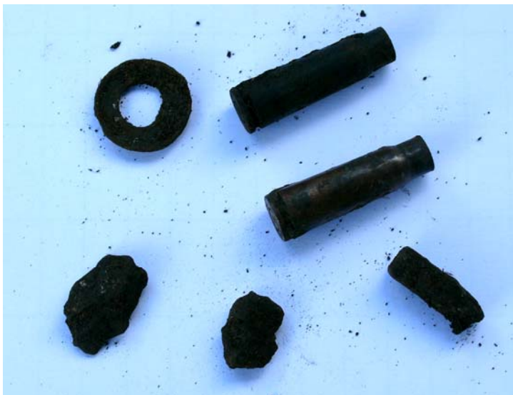
Figure 3 Indigenous clutter items used in the test: washer, two cartridges, bullet and two metal fragments
