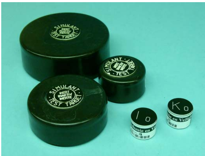
Figure 2a ITOP targets (left) and inserts Io and Ko (right).
