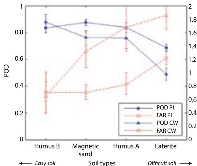
Figure 7. Performance of metal detectors in terms of POD (blue solid lines) and FAR (red dashed lines), separately calculated for pulse induction (PI, plotted with circles) and continuous wave (CW, plotted with triangles) detectors. Soil on the left side is considered to be easy and soil on the right side is considered to be difficult. The error bars show 95% confidence bounds.
