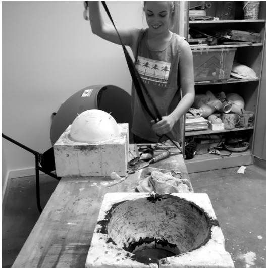
Figure 14: Strapping in the Styrofoam Ball and Texturizing the Concrete
