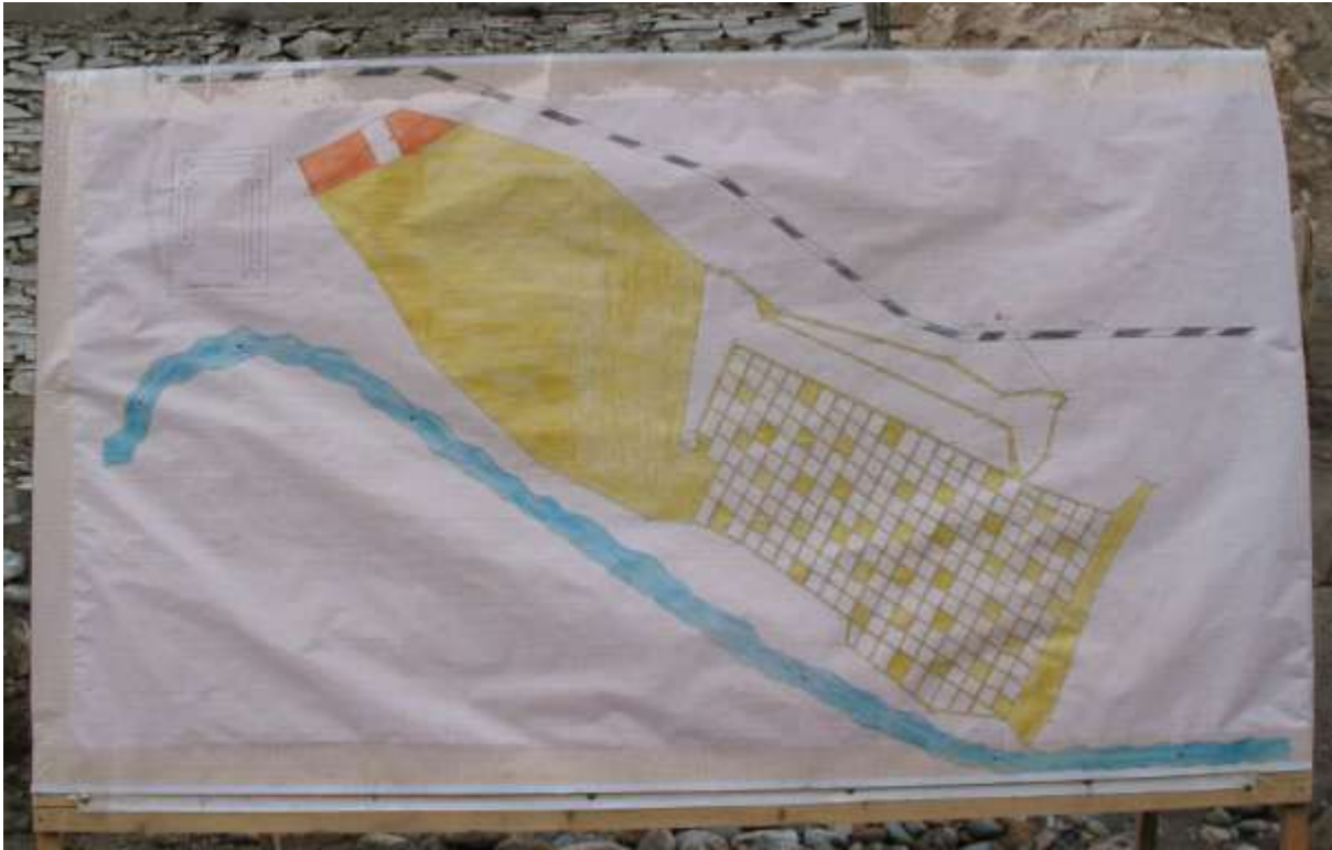
Figure 5. An FSD briefing map showing the different areas of their current task cleared by either full search by manual clearance (red), full search by dogs (yellow) and technical survey (chequerboard).
