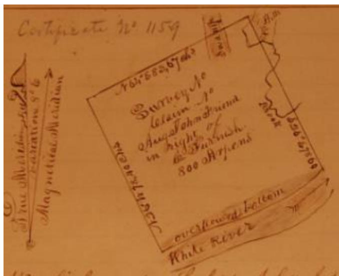
FIGURE 1: A typical plat from the Spanish Land Grant surveys conducted in 1805 until the mid-nineteenth century. This plat shows the White River, overflowed bottoms, and swamp.
