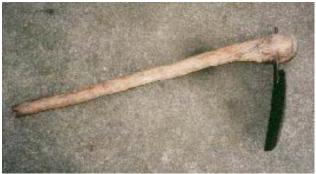
The use of the "enxada" (hoe) may seem inappropriate but in difficult ground conditions a similar tool is often found necessary. The length of the tool probably prevented serious hand injury - although its breaking into parts during the blast may have led to other injury.
