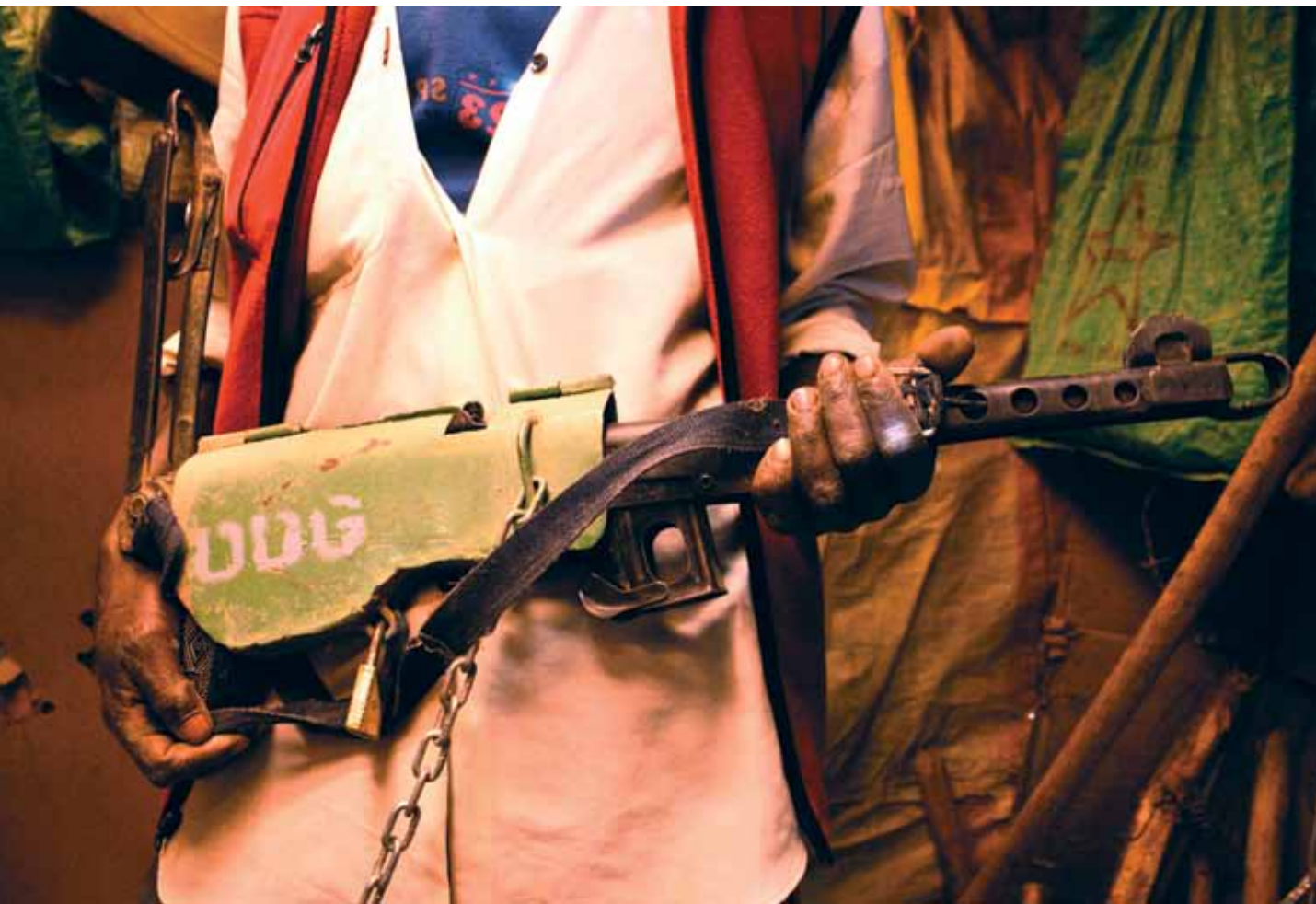
In collaboration with local communities, DDG has developed safe-storage devices, such as this gun clamp as well as boxes for pistols and ammunition. The devices are locked with a padlock and chained to the foundation of the owner's house, and they have proven very successful in preventing accidents and theft.
