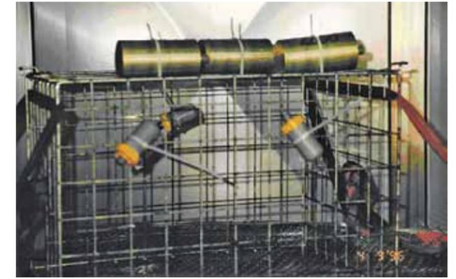
Images 1 and 2. Rain plant setup. All photos © Saab Bofors Dynamics Switzerland Ltd.
