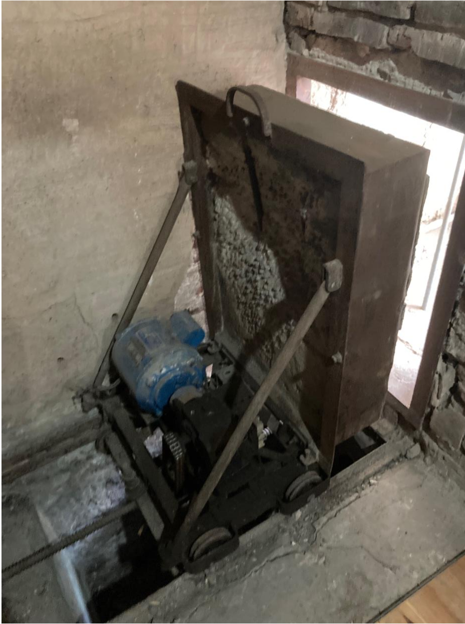
Figure 14. The machinery that moved the secret wall where the printing press was inside. See http://asociacionanahi.org.ar/ .
