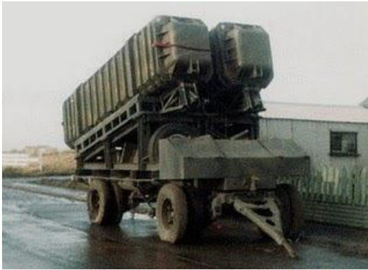
Figure4: Improvised launcher used by Argentines to engage British ships. Anti-ship missiles can also be a coastal threat. Taken from Mycity-Military forum.
