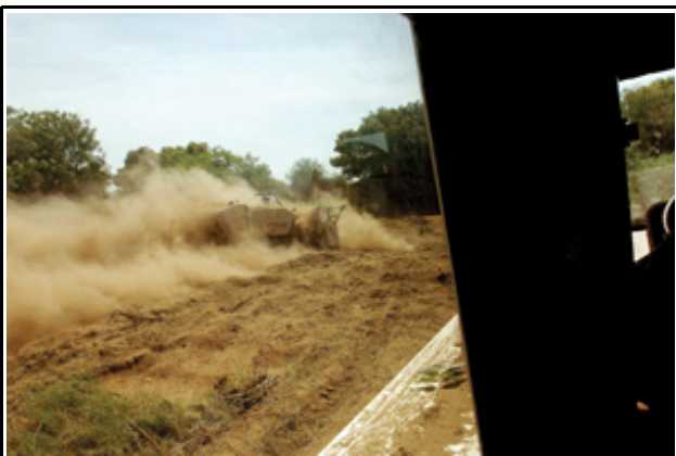
Engineers from ArmorGroup use MineWolf demining machines to clear AP landmines under a program coordinated by the UNMAO in consultation with the Government of Southern Sudan and other national and international actors. Approximately 2,000 AP mines
