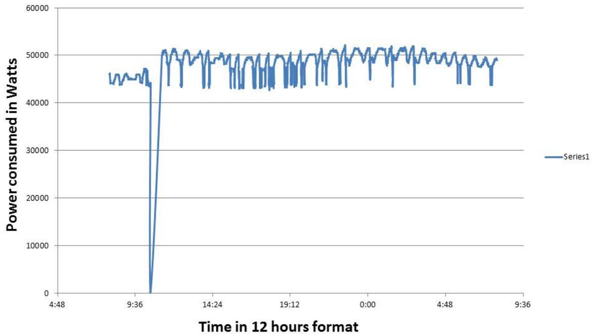
Figure 6.11 Power consumption per hour: Hibon day 1
