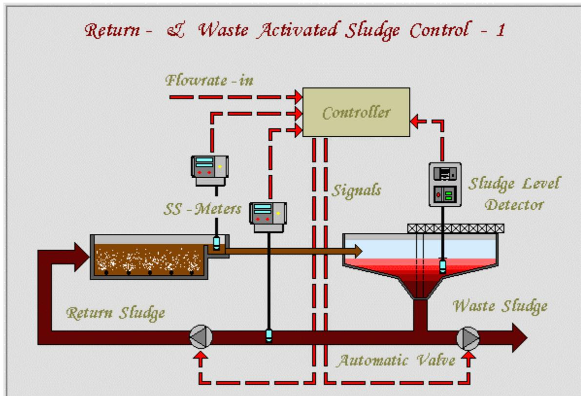
Figure 3.7 Return and Waste Activated Sludge Control Process [68]
