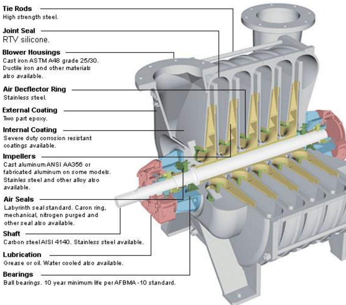
Figure 3.3 Pictorial representation of a Hibon multi- stage Centrifugal blower [64]
