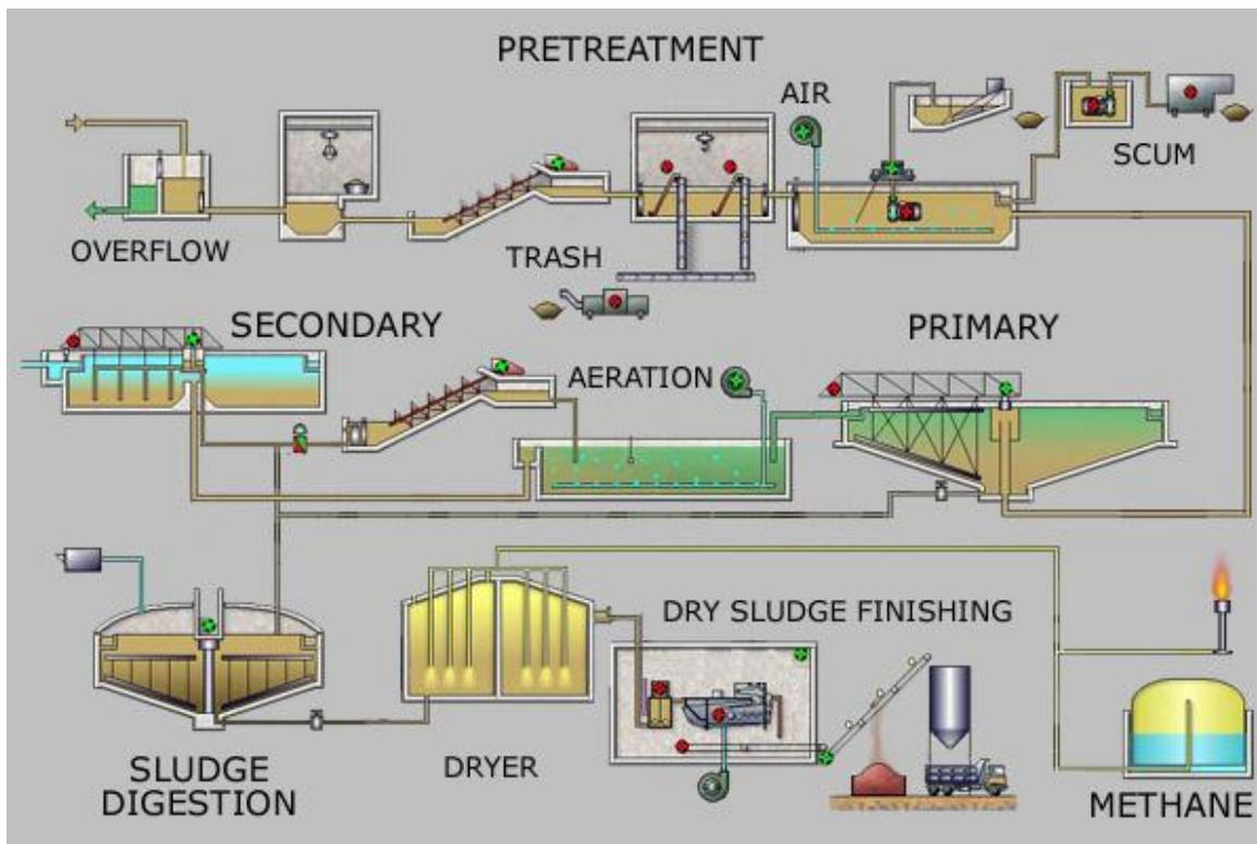
Figure 3.1 Process Flow Diagram for a typical large-scale treatment plant [62]
