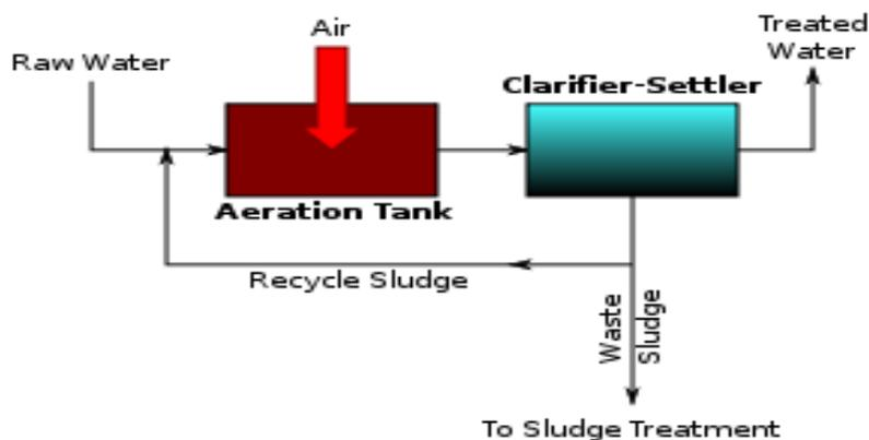
Figure 3.2 A generalized, schematic diagram of an activated sludge process [63]
