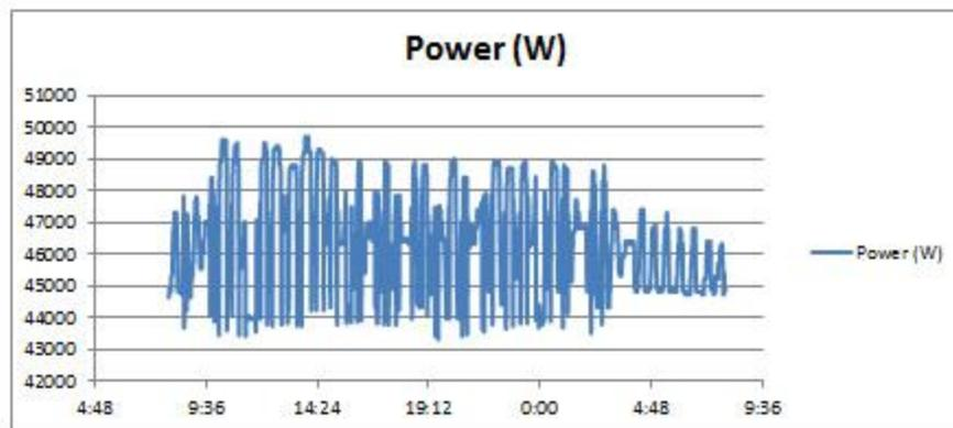
Figure 6.10 Power consumption per hour: Neuros Day 1 and 2.
