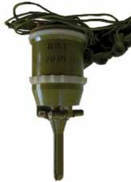
The Chinese Type 84 is a scatterable AT mine initiated by a magnetic influence fuze. All photos courtesy of the author.
