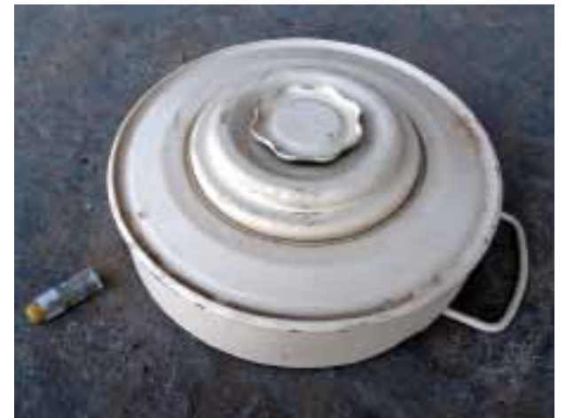
The Chinese Type 72 SP AT mine, with blast-resistant fuze to the left.
