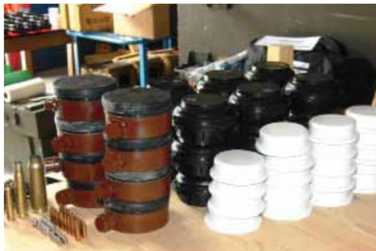
Objects used in the test. From left to right: metal clutter (ammunition belts, cartridges, bullets) and mine-like targets (Gyata-64, PPM-2, ERA calibration target). Photo courtesy of BWB.
