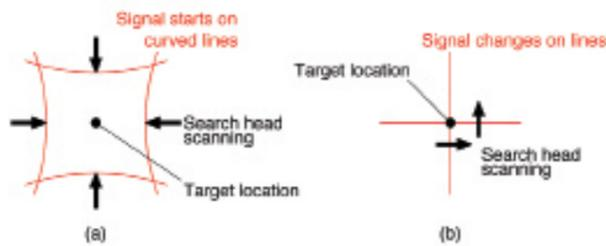
Figure 5. Pinpointing a target with (a) single-receive-coil detectors and (b) double-D coil detectors (reproduced from the STEMMD Lab Test report and Metal Detector Handbook).<sup>2,3</sup>
