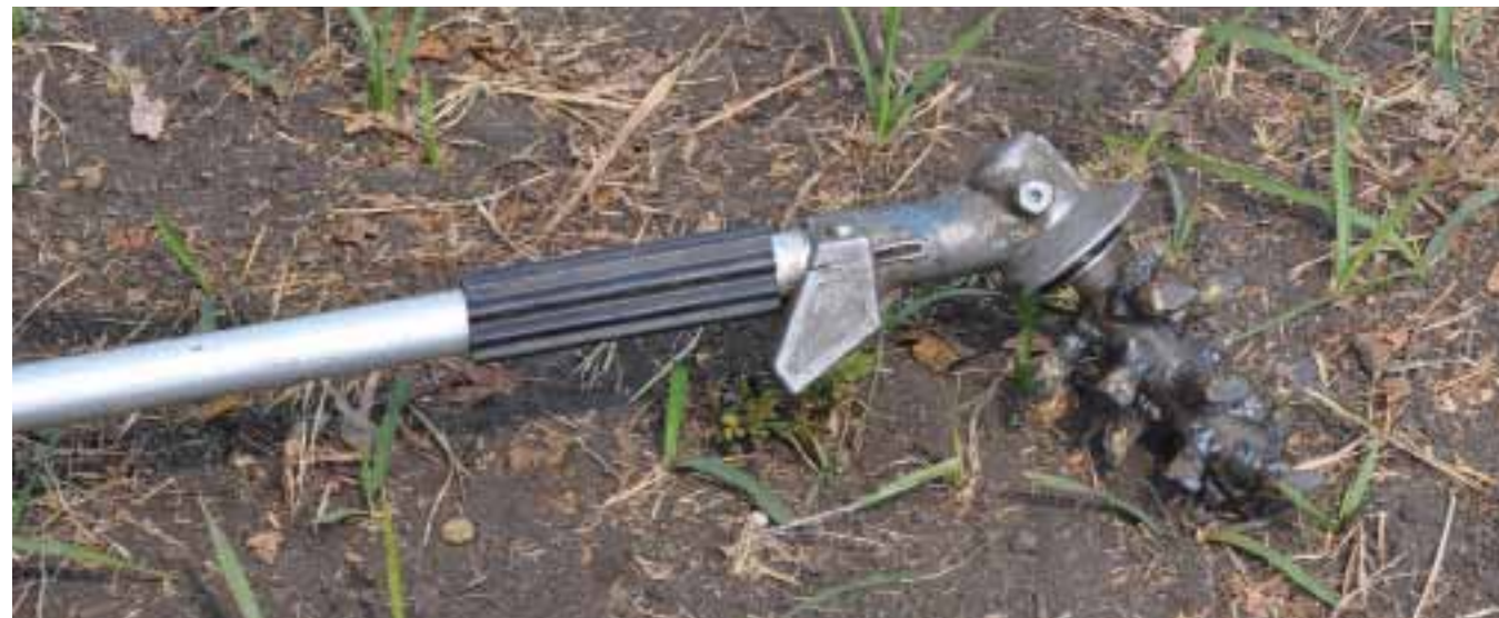
The basic design of the pineapple and the alignment of drill heads maximizes the potential for digging.
