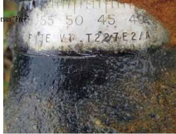
**Image 1** (left). U.S. BLU-26 submunition remains found at 55 cm. during Vung Ha clearance. **Image 2** (middle). U.S. BLU-61 submunition found in deep search excavation spoils during Vung Ha clearance. **Image 3** (right). U.S. 105-mm projectile with T-227E2 variable time fuze located at 1.5 m. deep in non-oxidizing layer, at Vung Ha clearance site.
