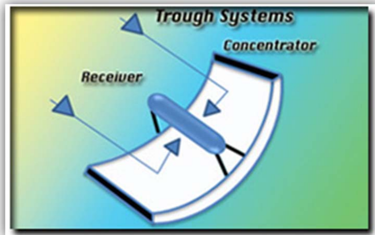
Figure 16. A schematic of a typical mirror for a linear CSP system. (Sandia National Laboratories)
