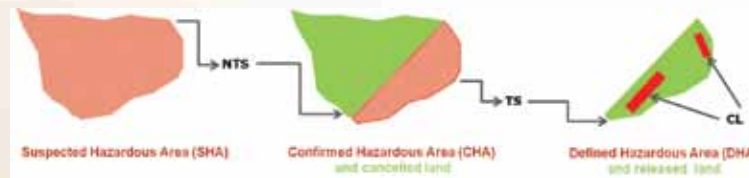
Figure 1. Toward better definition of the contamination through NTS and TS. Clearance is conducted on the DHA.
