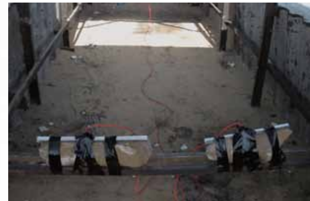
Six WP shells are prepared within demolition bins for demolitions with donor explosive charges attached. Photo courtesy of Kerei Ruru/UNMAT.
