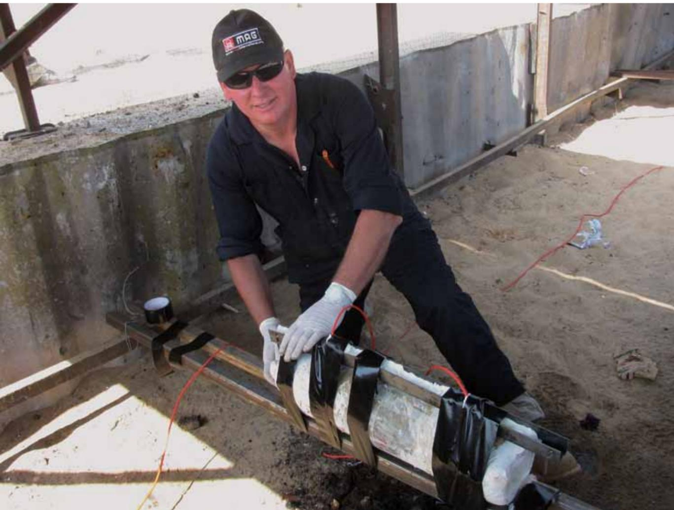
Leon Magnussen, MAG's Explosive Ordnance Disposal Technician, attaches an explosive shaped charge used to split 155-mm WP shells to expose WP.
