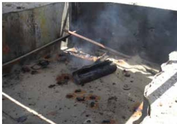
A 155-mm WP shell split by explosives exposes the white phosphorus sponges (black sponges seen to rear of shell). Photo courtesy of Mark Russell/UNMAT.
