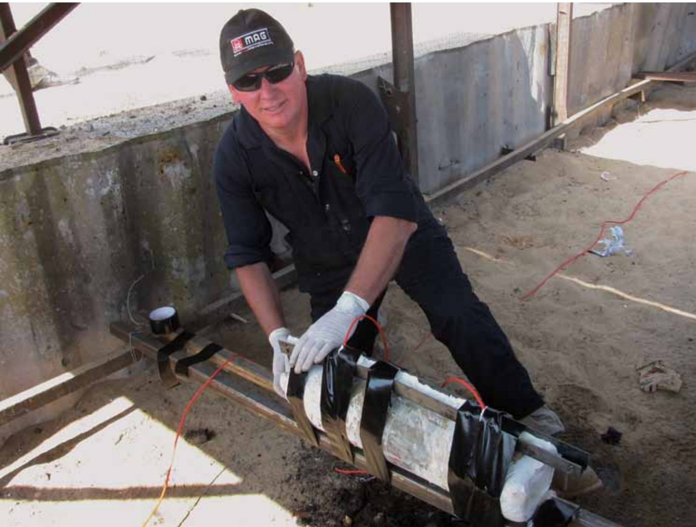
Leon Magnussen, MAG's Explosive Ordnance Disposal Technician, attaches an explosive shaped charge used to split 155-mm WP shells to expose WP. Photo courtesy of Kerei Ruru/UNMAT.
